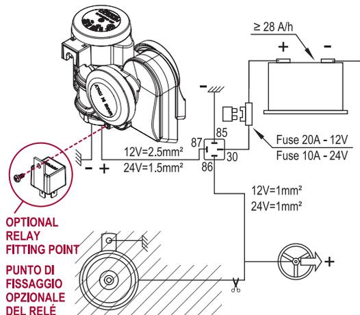
WIRING DIAGRAM WITH GROUND LEAD TO HORN BUTTON
